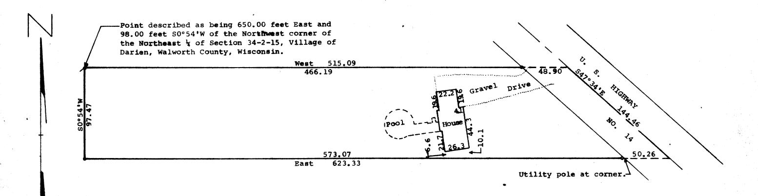
Scale -1" = 50'• = 1" Dia. Iron Pipe Found M = 3/4 Dia. Iron Pipe Found • = 3/4" Dia. Iron Pipe Set
